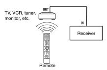
The remote sensor on the CONTROL S OUT component receives remote codes the same way as the remote sensor on this receiver. This is useful if you have placed this receiver in a rack, etc.
